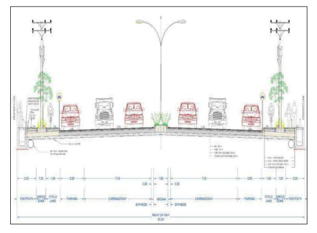
Figure 1–2. Schematic of 4 Lanes
